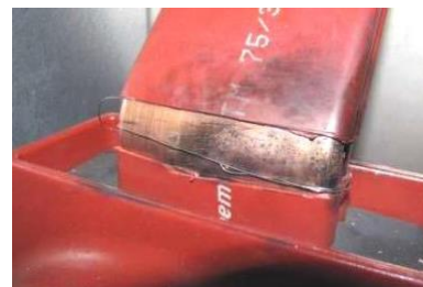
Figure 1 Point of Fault Initiation during AQD Testing
